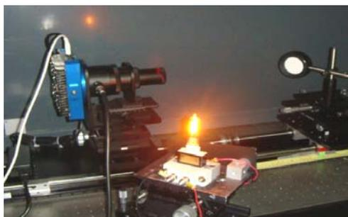
Figure 4 Spectral radiance calibration facility
